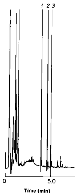
Fig. 2. Gas chromatograph-ECD chromatogram of 62.5 pg O 4 -ethyl- N 1-pentafluorobenzylthymine (3), with 16.5 pg each of lindane (1) and aldrin (2) as reference compounds
