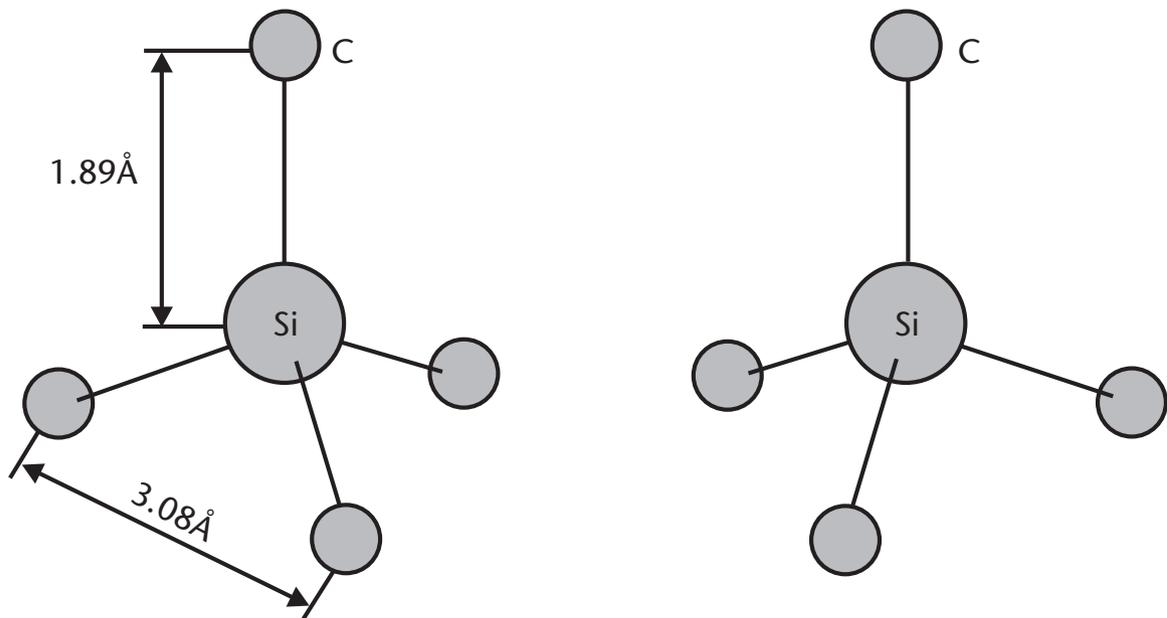
The characteristic tetrahedron building block of all silicon carbide crystals. Four carbon atoms are covalently bonded with a silicon atom in the centre. Two types exist. One is rotated 180° around the c-axis with respect to the other, as shown.
