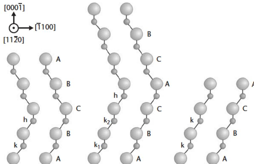
The three most common polytypes in silicon carbide viewed in the  $[11\bar{2}0]$  plane. From left to right: 4H-silicon carbide, 6H-silicon carbide, and 3C-silicon carbide; k and h denote crystal symmetry points that are cubic and hexagonal, respectively.
